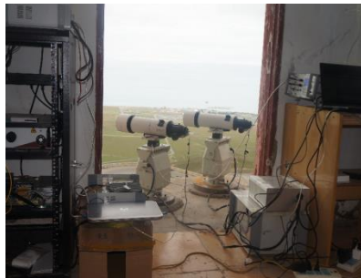
Fig. 2 field experiment of compound axis dual antenna structure
